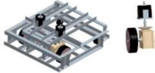
Figure 5 Base chassis assembled with motor, gear box and wheel
