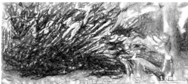
Figure 6. Cross sectional area of a broken specimen of V_f = 0\% showing multiple fracture with irregular pattern.
