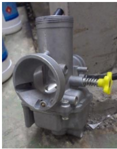
Gambar 3. Karburator Mikuni PE28 (diameter venturi \varnothing 50 mm)
