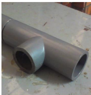
Gambar 5. Pipa manifold (PVC, D in 2.7 cm, D out 3.3 cm)
