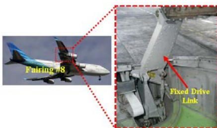
Fig.1 Location of installed Fixed Drive Link of Flap Track Fairing (canoe) #8 [1]
