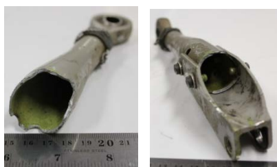
Fig.6 Fracture surface of component #3 from Fig.4. The Adjustable rod components were broken and split into two parts
