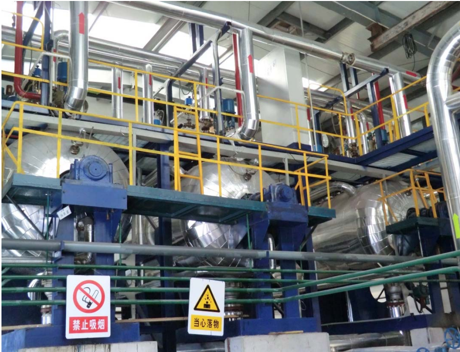
Three Reactors (7.8m 3 , 3MPa)
