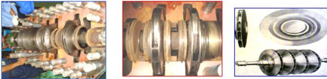
Gambar 2 : impeller pompa sentrifugal (Union Pump Chevron)
