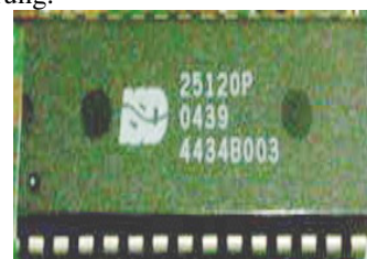
Gambar 3.2 IC ISD25120, 120 second audio recording and playback
